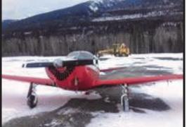
I never did the oil temps up on this trip making the oil pressure very high also the cylinder head temp ran very cold. A standard Canadian winter operational tip is use duct tape to cover the grill.
