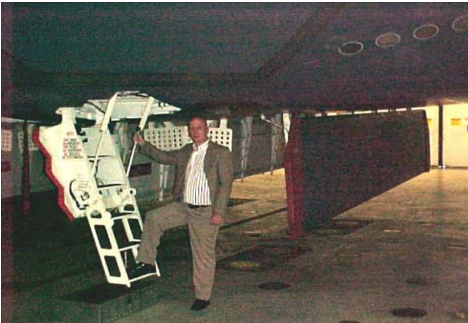
Mick ready to ascend. Note perforated plates to create turbulence ahead of the bomb bay.
