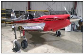
Serial #58, GC-1A converted to a GC-1B. Past Oshkosh Lindy Award winner. Powered by a 210 HP Continental engine, equipped with a Nagel sliding canopy, sticks, and retractable tailwheel. Smooth skinned, flush riveted, and a recent leather interior installed with Cessna 152 seats.
