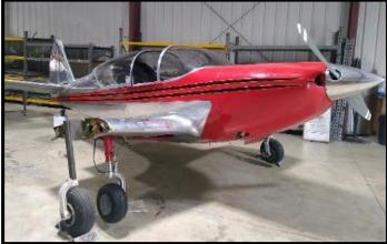
Serial #58, GC-1A converted to a GC-1B. Past Oshkosh Lindy Award winner. Powered by a 210 HP Continental engine, equipped with a Nagel sliding canopy, sticks, and retractable tailwheel. Smooth skinned, flush riveted, and a recent leather interior installed with Cessna 152 seats.
